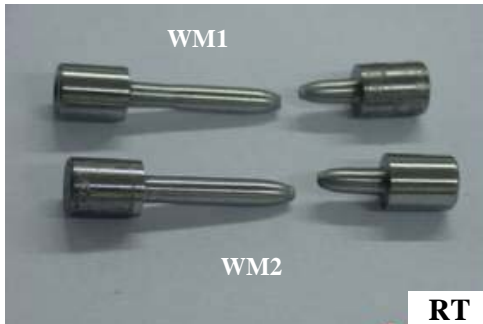
Fig. 4: Tensile tested cross-weld specimens showing presence of double necking in WM1 weldment and single necking in WM2 weldment
