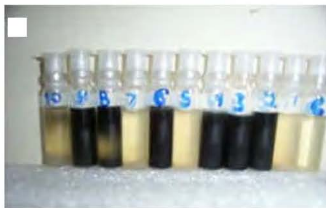
Figure 2. The precipitation of FeS due to activity of SRB containing different soap–detergent solution (as the only carbon source) modified media after 5 days of incubation with mud-leached water from tubewell-1, and control (C, extreme right).
