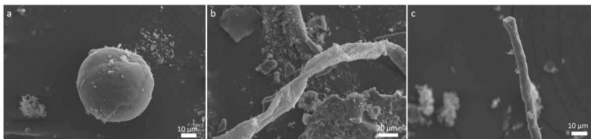
Figure 1. SEM images of the residues obtained after shock processing glycine. (a) globule structure, (b) fine filamentous thread feature and (c) cylindrical fibril feature.
