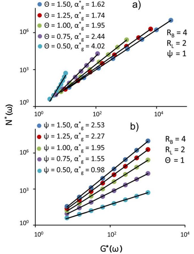
**Figure 3.**  $N^*(\omega)$  versus  $G^*(\omega)$  curves for different values of  $\Theta$  and  $\Psi$ : when (a)  $\Psi = 1$  and (b)  $\Theta = 1$ . In all cases,  $R_B$  and  $R_L$  were 4 and 2, respectively, and  $L_{\Omega}$ ,  $q$ , and  $c$  are equal to 1. It can be observed that the power law exponent  $\alpha_g^*$  is increasing with  $\Psi$  but decreasing with  $\Theta$ .
