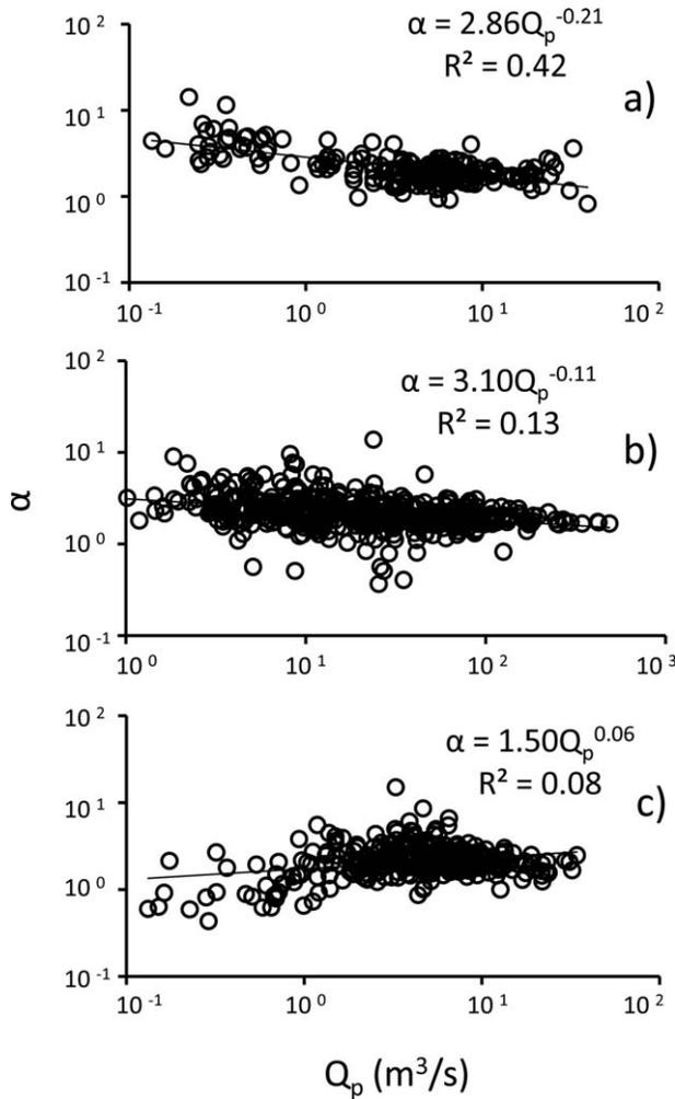
**Figure 5.** The power law exponent ( $\alpha$ ) of a recession curve versus its recession peak ( $Q_p$ ) curve ( $\alpha \propto Q_p^{-\sigma}$ ) for: (a) Bear (USGS id: 03076600; area = 126.65 sq km), (b) Tunkhannock (USGS id: 01534000; area = 991.75 sq km), and (c) Paluxy (USGS id: 08091500; area = 1061.90 sq km). Positive value of sigma indicates  $ds/dl$  increasing with  $l$ , and vice versa.
