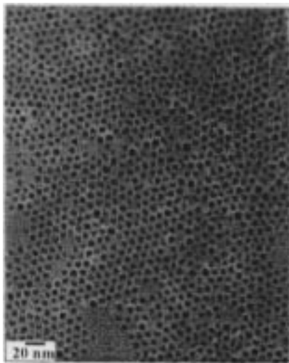
Figure 3. TEM micrograph showing arrays of Pd 561 Ni 3000 Pd 1500 nanoparticles coated with octylamine.
