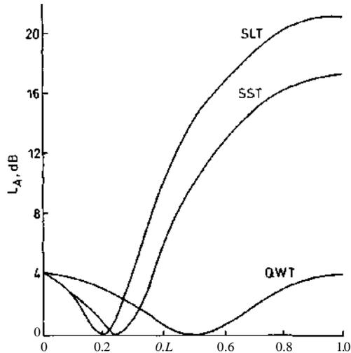
Fig. 2 Matching characteristics of QWT, SLT and SST for  $r = 8$
