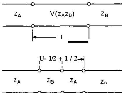
Fig. 1 Short-length transformer (SLT)
