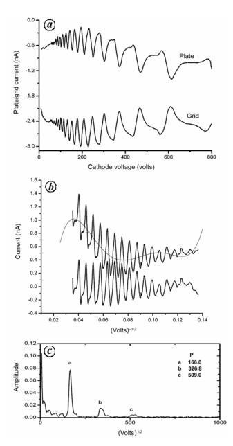
**Figure 2.** Plate/grid current variation as a function of electron energy. *a*, Observed plate and grid current responses. *b*, Plate current response of (*a*) replotted as a function of  $\mathcal{E}^{-1/2}$ . This yields equally spaced peaks. *c*, Fourier plot of curves (*b*) showing a dominant frequency peak and two non-dominant peaks corresponding to second and third harmonics.
