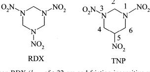
than RDX ( $h_{50\%}$  of >32 cm and friction insensitive up to 17-18 kg load), which may be due to the presence of a C-NO<sub>2</sub> group in the molecule in place of N-NO<sub>2</sub> group in RDX.
