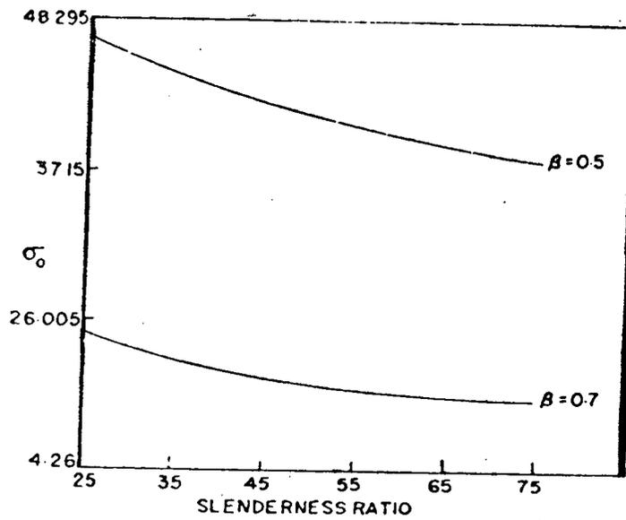
FIG. 8. CRITICAL LOADS OF SHORT COLUMNS
