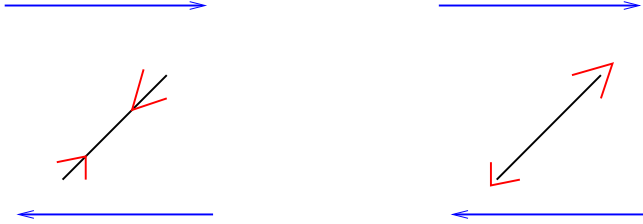
FIG. 8: How activity modifies viscosity: Shear orients filaments; the permanent force dipoles pull back, if contractile, and push out, if extensile, on the flow.
