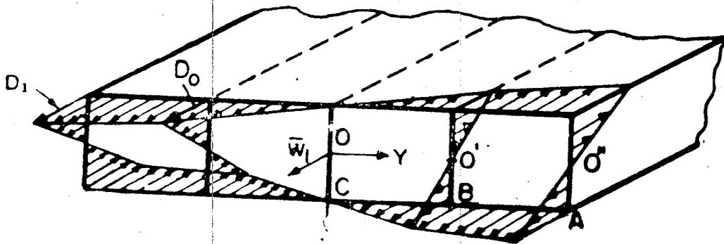
Fig. 5 Distribution of  $\bar{w}_1$  in Four-Cell Tube
