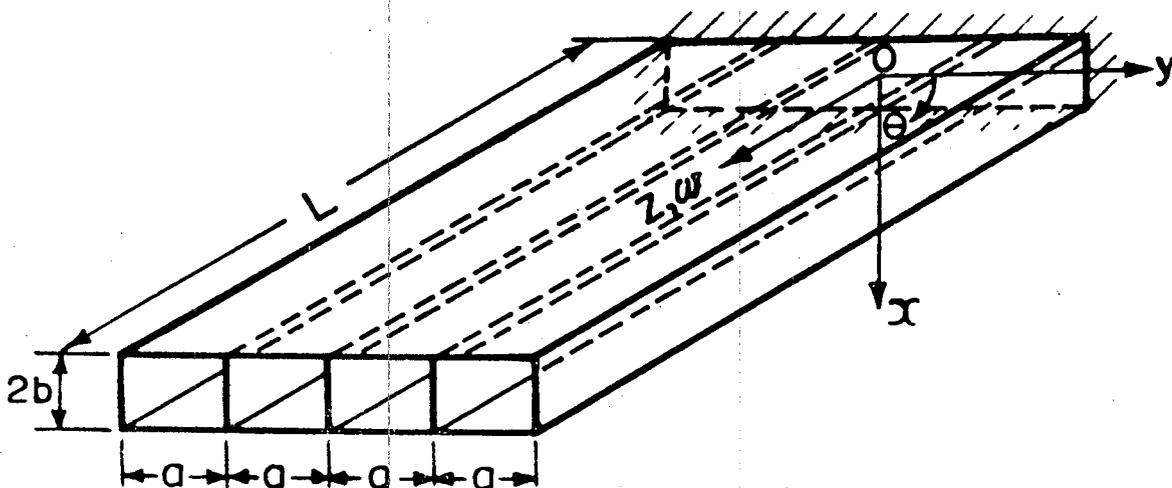
Fig. 1 A Cantilever Four-Cell Tube
