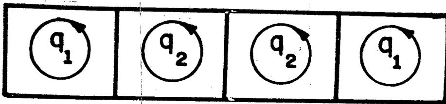
Fig. 7 Shear flows in Doubly—Symmetric Four—Cell Tube
