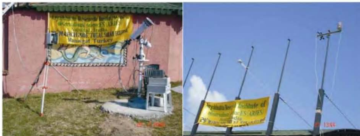
Figure 2. Photograph shows our experimental set-up. (Left panel) Telescope used to make observations of the solar eclipse. The data logger for the mini weather station placed on a tripod is also shown. (Right panel) Different sensors of the mini weather station.
