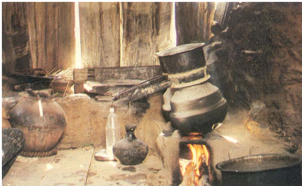
Plate 1—Traditional distillation unit for Soor
