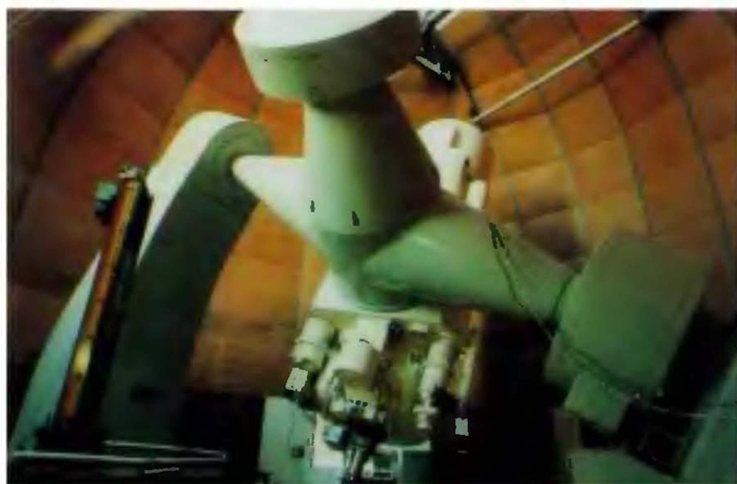
Figure 2. A view of the 104-cm Sampurnanand telescope of UP State Observatory, Nainital. CCD imaging unit is mounted at the Cassegrain focus of the telescope.
