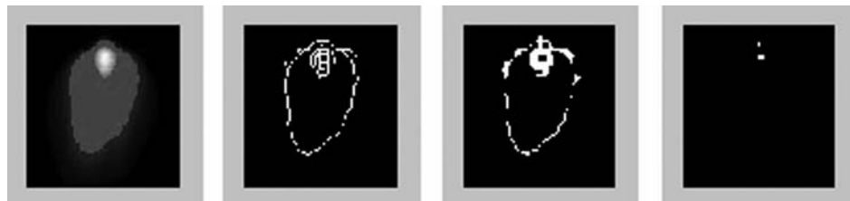
Fig. 8—Gray scale, image, edge detected, region filled and hotspot isolated images for depth of penetration (60 %) thermograph
