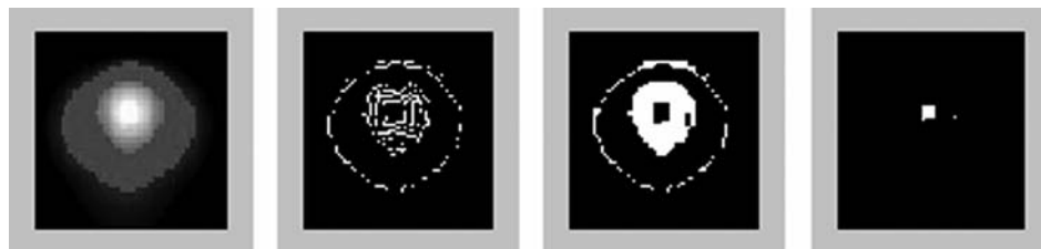
Fig. 7—Gray scale, image, edge detected, region filled and hotspot isolated images for depth of penetration (80 %) thermograph
