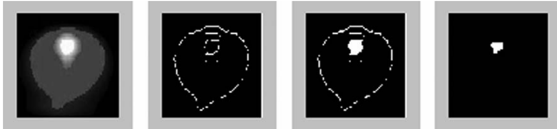
Fig. 6—Gray scale, image, edge detected, region filled and hotspot isolated images for depth of penetration (100 %) thermograph
