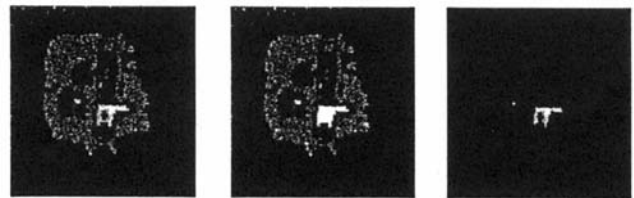
Fig. 13—Appended, region filled and output image for gauge shaped tungsten inclusion detection by region growing
