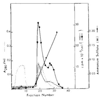
Figure 45. Phosphocellulose column chromatography. A linear gradient elution was carried out with increasing concentration of ammonium sulfate from 10 mM to 200 mM in Buffer B; 1 ml fractions were collected. Assay of DNA polymerase was carried out in presence (—) and absence (---) of 100 mM ammonium sulfate.
