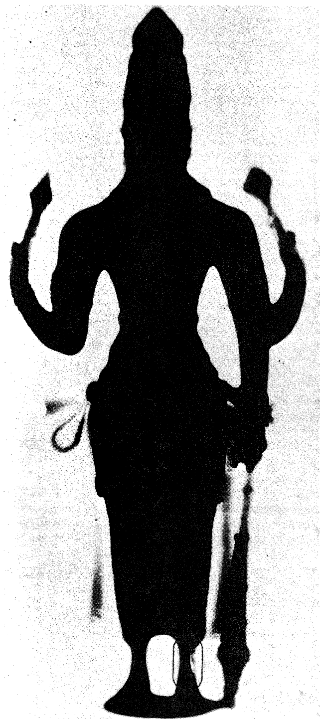
Figure 3. Radiograph showing the repair in the leg region of one of the idols (9th century).
