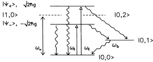
FIG. 1. Schematic representation of various energy levels and the transitions. The solid lines give the two pathways for the absorption of external photon. The wavy lines give the cavity induced decays.
