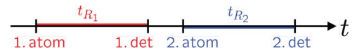
Fig. 2. (Color online) Schematic representation of the scenario that the first scattered photon is detected before the second photon is emitted. In this case the two photons do not exist in the same interval of time.
