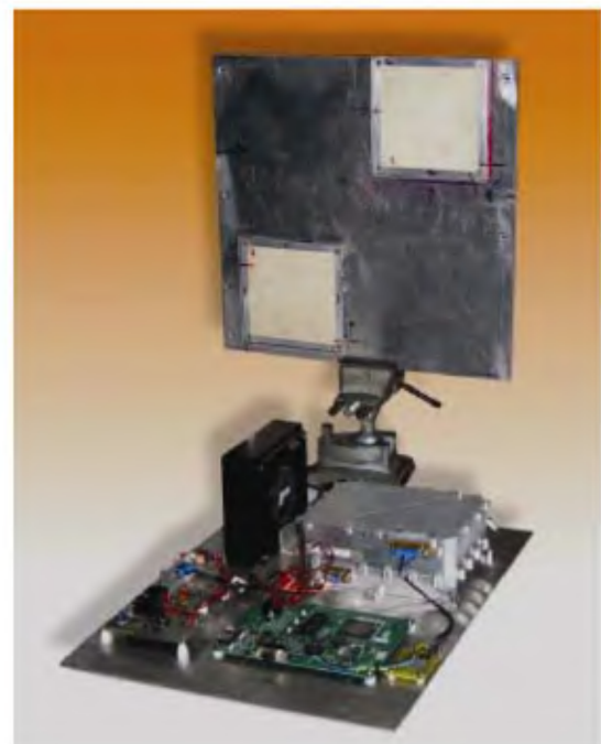
Figure 5. Moon Impact Probe radar altimeter: aircraft test setup.
