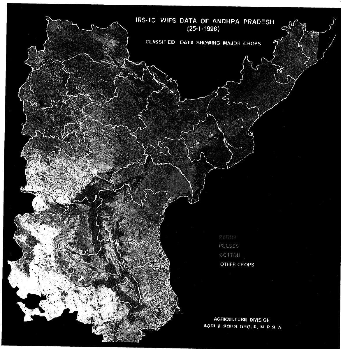
Figure 2. Two-band false colour composite (FCC, colour assignments are red: NIR band-B4, green & blue: red band-B3) of WiFS scene (25 January 1996) overlaid with district boundaries and distribution of major crops (paddy, pulses, cotton and other crops) in Andhra Pradesh.
