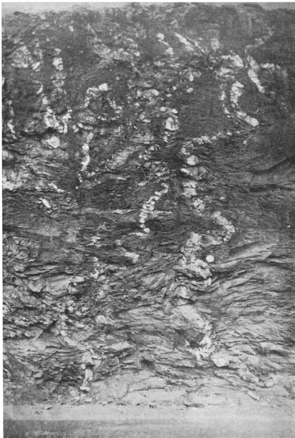
Concentrically folded quartz veins in phyllite showing 40–42% buckle shortening.
