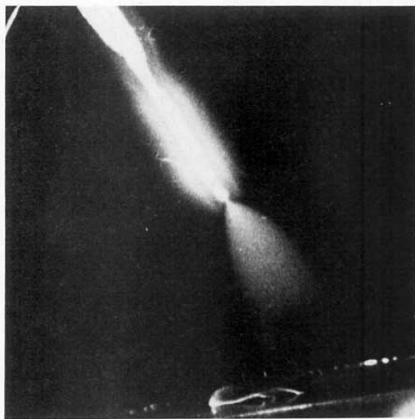
FIG. 2. Smoke of very fine water droplets coming off the tip of a wet leaf of Ellitaria plant when a positive d.c. voltage of 5.0 kV is applied to the plant and a grounded plate is kept 2.5 cm below the tip.
