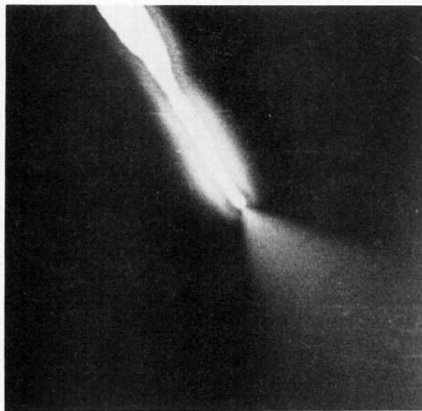
FIG. 1. Smoke of very fine water droplets coming off the tip of a wet leaf of Ellitaria plant when a positive d.c. voltage of 9.5 kV is applied to the plant.
