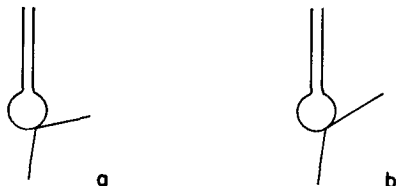
FIG. 3. Trajectories of spheres of 200 \mu radii before and after collision with a sphere of 2 \text{ mm} radius in electric fields of 1.9 \text{ kV cm}^{-1} , a., and 2.0 \text{ kV cm}^{-1} , b.
