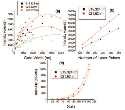
Figure 4. Variation in LIBS signal with (a) gate width, (b) number of laser pulses and (c) gain.
