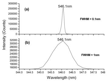
Figure 3. Spectral resolution of (a) echelle spectrograph and (b) Czernyturner spectrograph.
