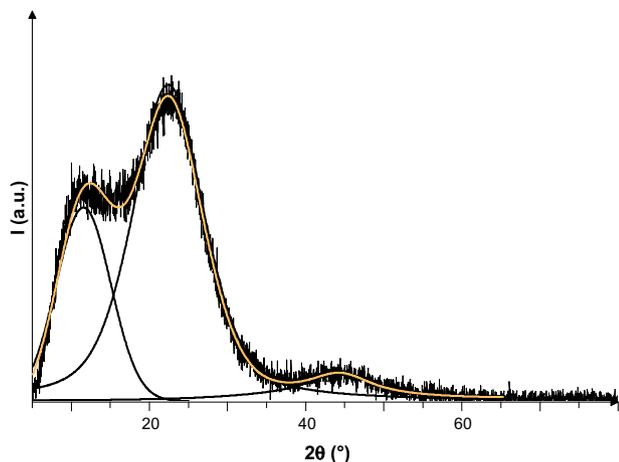
**Fig. 5 – X-ray powder pattern of the carbon material after subtraction of the background modeled by a 7-points Bezier function. The three diffraction lines are fitted by a pseudo-Voigt function.**
