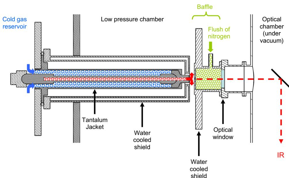
Fig. 1 – Circumstellar carbon analogues reactor. The source is coupled to a FT-IR spectrometer through its spectroscopy interface.
