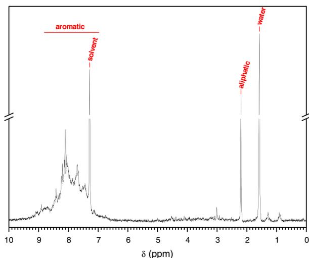
Fig. 3 – Proton NMR spectrum of the soluble fraction of the carbonaceous material produced by pyrolysis of acetylene in the porous graphite reactor.
