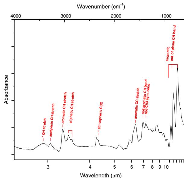
Fig. 4 – Mid resolution ( $4\text{ cm}^{-1}$ ) Fourier transform infrared absorption spectrum of the carbonaceous material mixed with KBr powder and pressed into a pellet.
