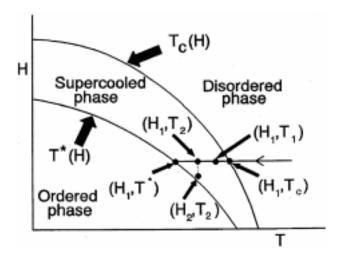
**Figure 1.** We show a schematic of the phase transition line  $T_{\rm C}(H)$  and the stability limit  $T^*(H)$  for the supercooled state:  $(H_1, T_1)$  and  $(H_1, T_2)$  indicate supercooled states when vortex matter is cooled in a field  $H_1$ . See text for details.
