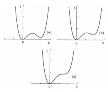
**Figure 3.** We show schematic free energy curves for (a)  $T = T_3 > T_{\rm C}$ , (b)  $T = T_4 > T_3$  and (c)  $T = T^{**}$ . The ordered state sits in a local minimum and is stable against infinitesimal fluctuations for  $T_{\rm C} < T < T^{**}$ .
