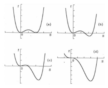
**Figure 2.** We show schematic free energy curves for (a)  $T = T_{\rm C}$ , (b)  $T = T_1 < T_{\rm C}$ , (c)  $T = T_2 < T_1$  and (d)  $T = T^*$ . The disordered state sits in a local minimum and is stable against infinitesimal fluctuations for  $T_{\rm C} > T > T^*$ . This local minimum becomes shallower as T is lowered below  $T_{\rm C}$  and the disordered state at  $T_2$  is unstable to a smaller fluctuation energy than at  $T_1$ .
