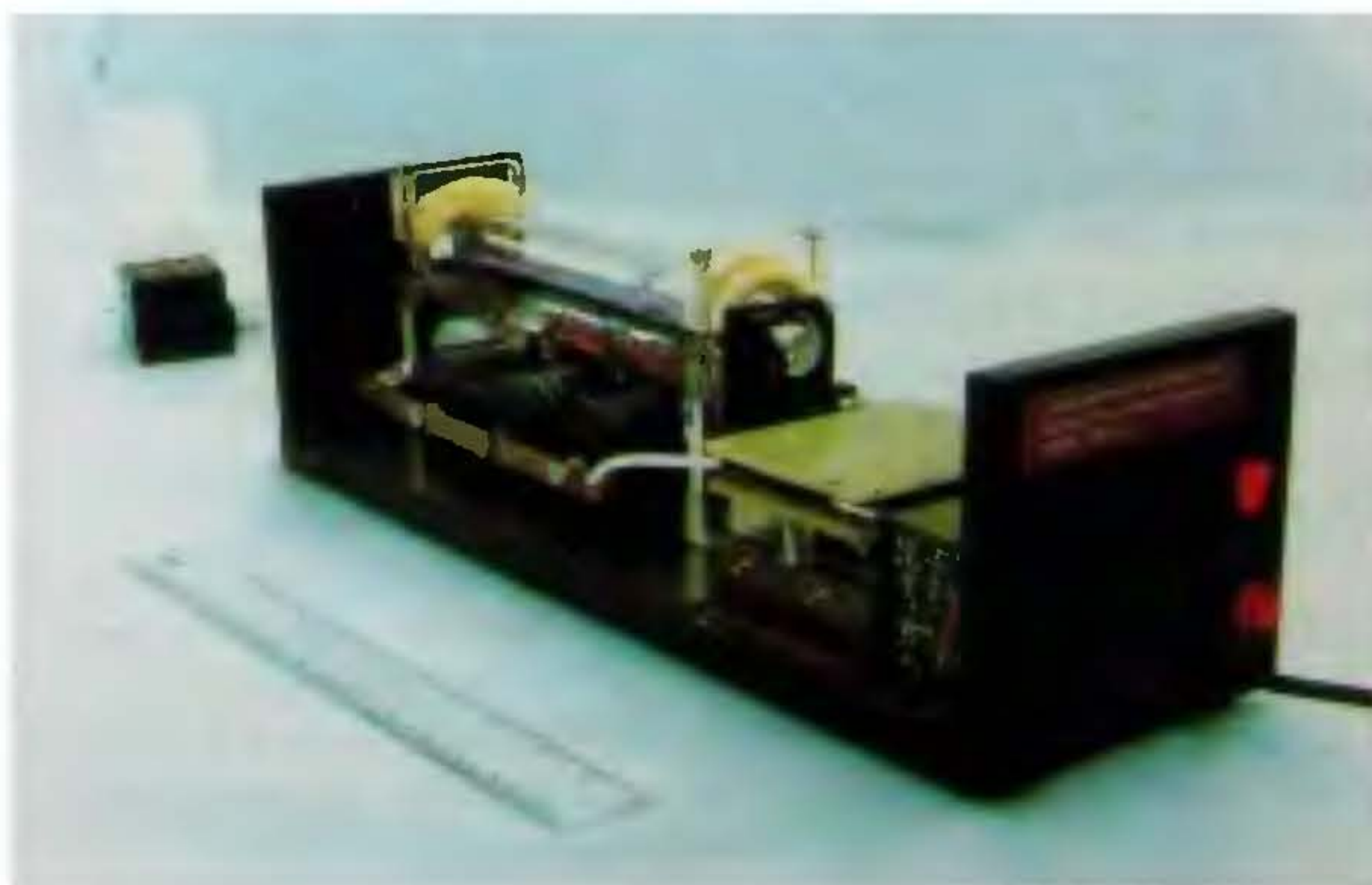
Figure 3. A sealed N 2 laser developed at CAT.
