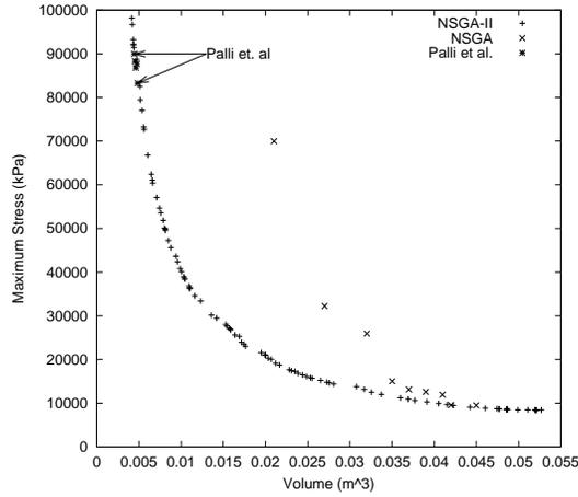
**Fig. 2.** Optimized solutions obtained using the NSGA-II and NSGA for the two-bar truss problem. Five solutions found in [8] are also shown for comparison.
