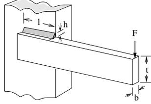
**Fig. 6.** The welded beam design problem. Minimizations of cost and end deflection are two objectives.
