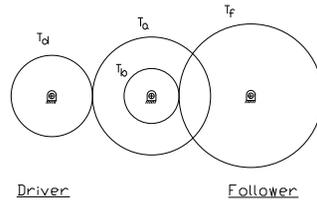
**Fig. 3.** A compound gear train is shown.
