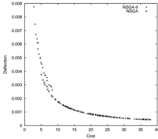
**Fig. 7.** Non-dominated solutions obtained using NSGA-II and NSGA for the welded beam design problem.
