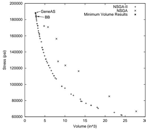
**Fig. 5.** Optimized solutions obtained using NSGA-II and NSGA for the spring design problem. Previously found solutions with GeneAS and branch-and-bound (BB) methods are also shown.
