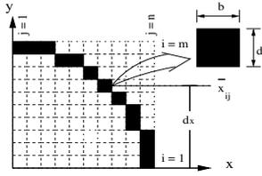
**Figure 1: Quadrant of a symmetric rectangular cross-section**
