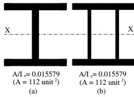
**Figure 5: Optimum cross-sections for Case-1, obtained from single objective minimization of  $A/I_x$**
