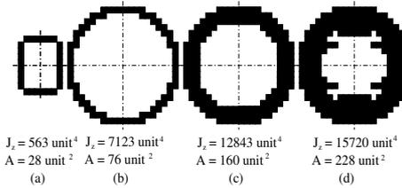
Figure 10: Optimum cross-sections for Case-3
