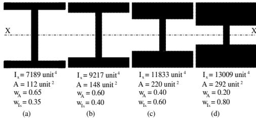
**Figure 6: Optimum cross-sections for Case-1, obtained from single objective minimization of  $w_1 A/A_{max} - w_2 I_x/I_{x,max}$**
