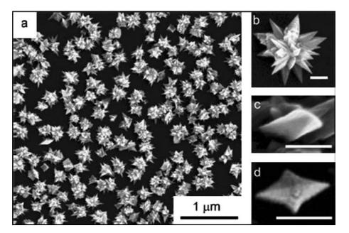
Fig. 23. SEM images of platinum nanothorns. (a) Large area SEM image; (b) high magnification SEM image of a platinum nanothorn; (c) side view of a nanothorn; (c) top view of a nanothorn. The scale bar in (b), (c), and (d) is 100 nm. Reproduced with permission from Reference (226). Royal Society of Chemistry, Copyright (2006).
