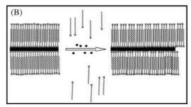
Fig. 9. Cartoon representation of (A) 3-D morphology showing (111) end-faces and (100) side-faces. (B) Illustration of 'zipping' mechanism for the formation of the bilayer of CTAB (squiggles) on the NR (black rectangle) surface may assist NR formation as more gold ion (black dots) is introduced. Reproduced with permission from Reference (170). American Chemical Society, Copyright (2005 and 2003).
