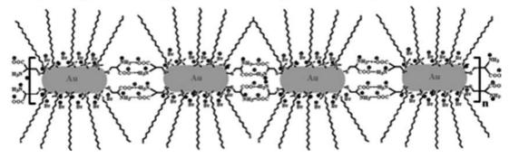
Fig. 28. (A) Schematic of the general mechanism of GNR nanochain formation due to electrostatic interaction due to cysteine and glutathione. Reprinted with permission from Reference (262). American Chemical Society, Copyright (2005).
