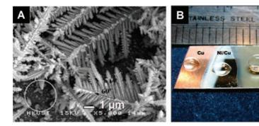
Fig. 42. (A) SEM image of Ag crystallites. (B) Photograph of water droplets on the Ag dendritic film surface, Ni surface, and Cu surface. All surfaces were modified with n-dodecanethiol. Reproduced with permission from Reference (227). American Chemical Society, Copyright (2008).
