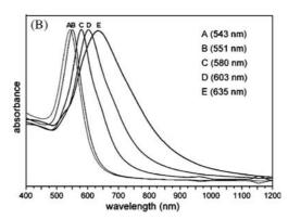
Fig. 18. (A) SEM image of the octahedral gold nanocrystals. The imaged regions show extensive self-assembled structures. (B) UV-vis absorption spectra of octahedral nanoparticles of different sizes. Maximum absorbance of the spectra has been normalized. Reproduced with permission from Reference (204). American Chemical Society Copyright (2008).
