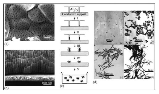
Fig. 24. (A and B) FESEM images of an alumina membrane. (C) Schematic representation of the successive stages during formation of GNRs via the template method. (D) TEM micrographs of GNRs obtained by the template method. Reproduced with permission from Reference (234). American Chemical Society, Copyright (2000).
