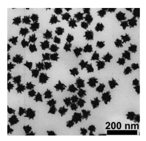
Fig. 7. TEM image of Au nanostars synthesized through reduction of HAuCl<sub>4</sub> in a PVP/DMF mixture, in the presence of preformed Au seeds, using 10 mM PVP. Reproduced with permission from Reference (42). Institute of Physics, Copyright (2006).
