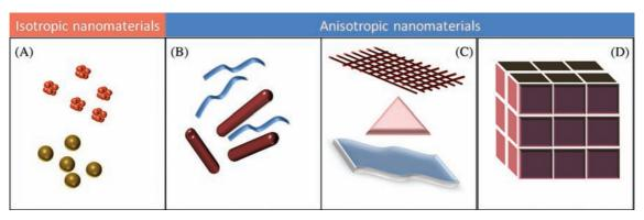
Fig. 1. Various kinds of nanomaterials. (A) 0D spheres and clusters. (B) 1D nanofibers, wires, and rods. (C) 2D films, plates, and networks. (D) 3D nanomaterials.
