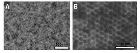
Fig. 30. TEM images of assemblies of hydrophobic GNRs arranged (A) parallel (B) perpendicular to substrate. Reprinted with permission from Reference (267). American Chemical Society, Copyright (2007).
