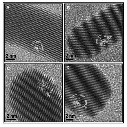
Fig. 10. HRTEM images of NRs formed using different seed particles: (A) Fe (bcc), (B) Cd (hcp), (C) Sb (trigonal), and (D) In (tetragonal). Although the metals are of different crystal structures, the GNRs formed are fcc. Reproduced with permission from Reference (173). Springer-Netherlands, Copyright (2010).
