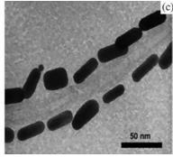
Fig. 31. TEM images of Au NRs (average aspect ratio 2.94), assembled on MWNTs (average diameter 30 nm) at various magnifications. Reproduced with permission from Reference (271). Wiley-VCH, Copyright (2005).
