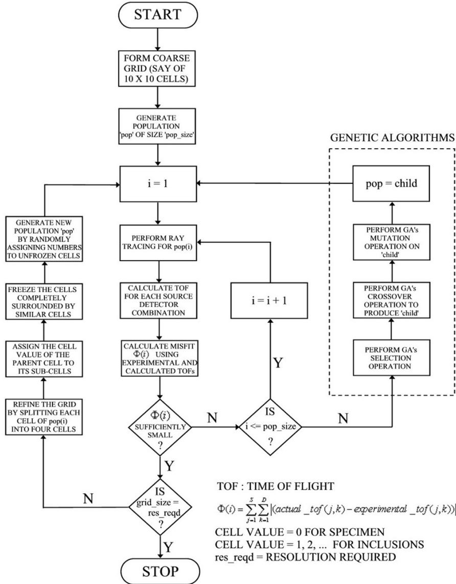
Figure 3. Flowchart of the GA based reconstruction algorithm
