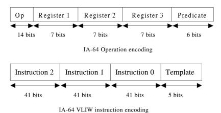
Each VLIW instruction (*bundle* in IA-64 terminology) consists of 128 bits. This means that each VLIW instruction can accommodate three 41 bit operations leaving five bits of the instruction encoding free. These five bits are used for the template which assists in decoding and routing the instructions and also the location of stops that mark the end of a group of instructions that can execute in parallel.
