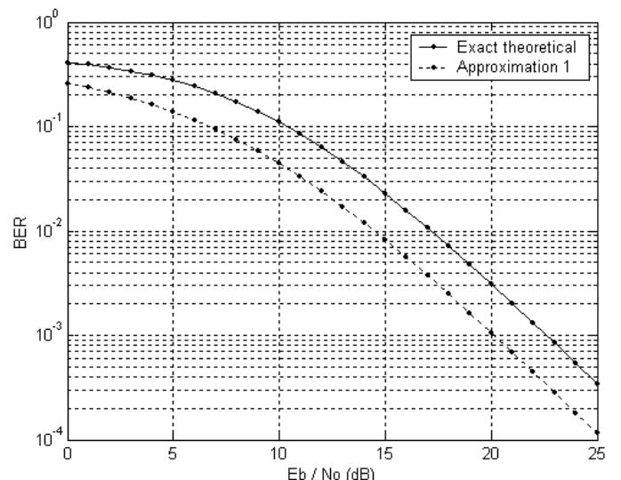
Fig. 5. Verification of the approximate analytical BER formula for DCSK in Rayleigh fading channels with 2-fold diversity
