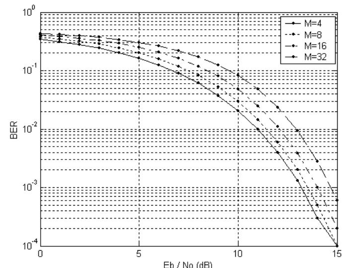
Fig. 2. Theoretical DCSK performance in AWGN channels.
