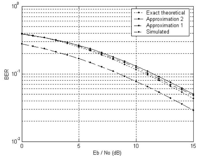
Fig. 3. Comparing different analytical BER expressions with simulated values for DCSK in Rayleigh fading channels (M=8)
