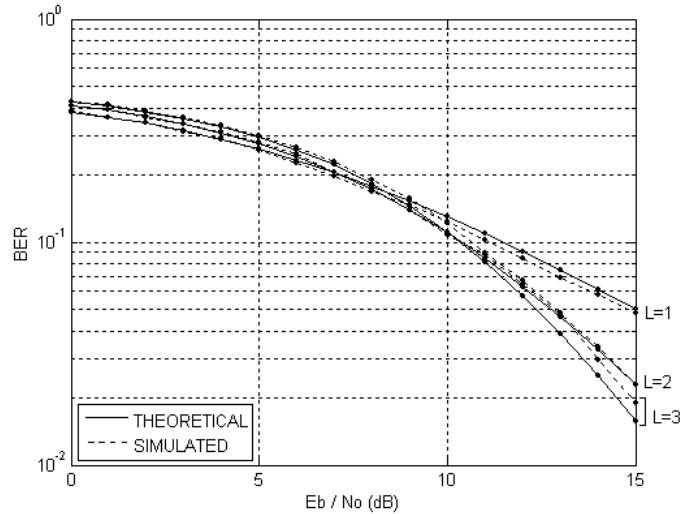
Fig. 4. Comparison of theoretical and simulated performances of DCSK in Rayleigh fading channels with diversity ( $M=8$ )
