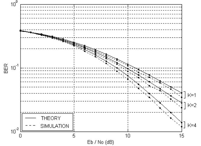
Fig. 6. Comparing simulated and theoretical performances of DCSK over 2-ray Ricean fading channels (M=8)
