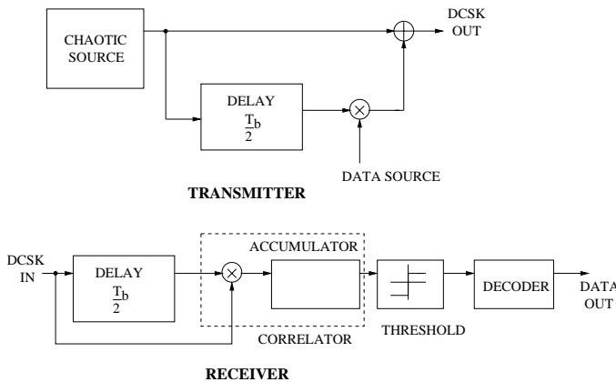
Fig. 1. DCSK transmitter and receiver structures.
