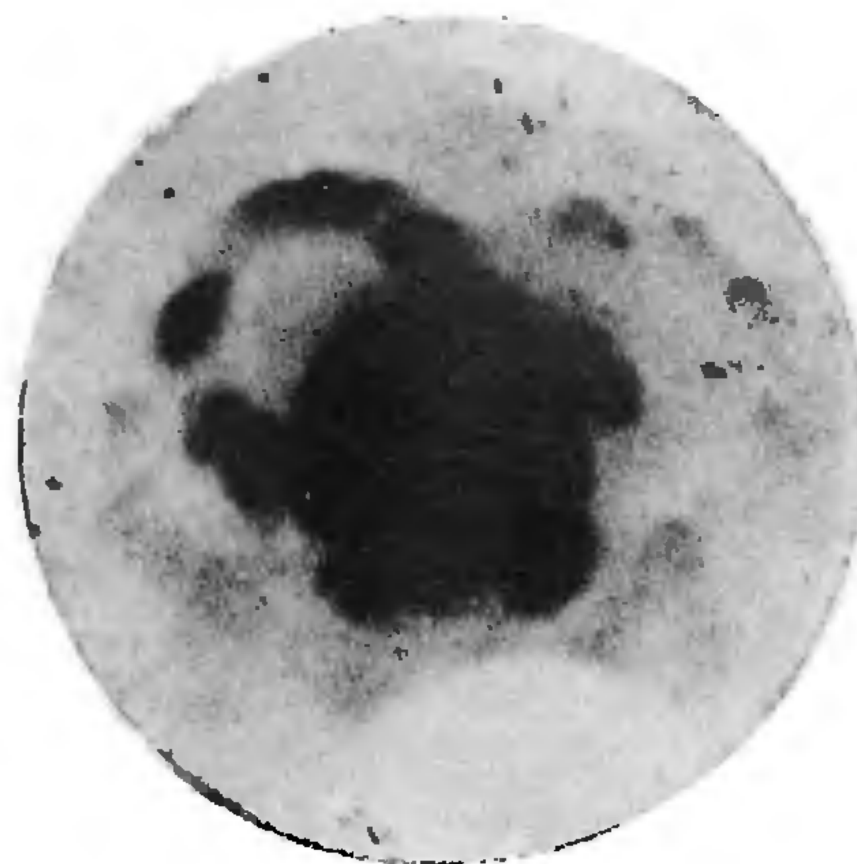
Figure 3. The first X-ray diffraction photograph recorded on samples of \text{CuSO}_4 \cdot 5\text{H}_2\text{O} . The ring of spots proved that X-rays were waves. (Source: Protein Crystallography (eds Blundell and Johnson), Academic Press, London, 1976.)
