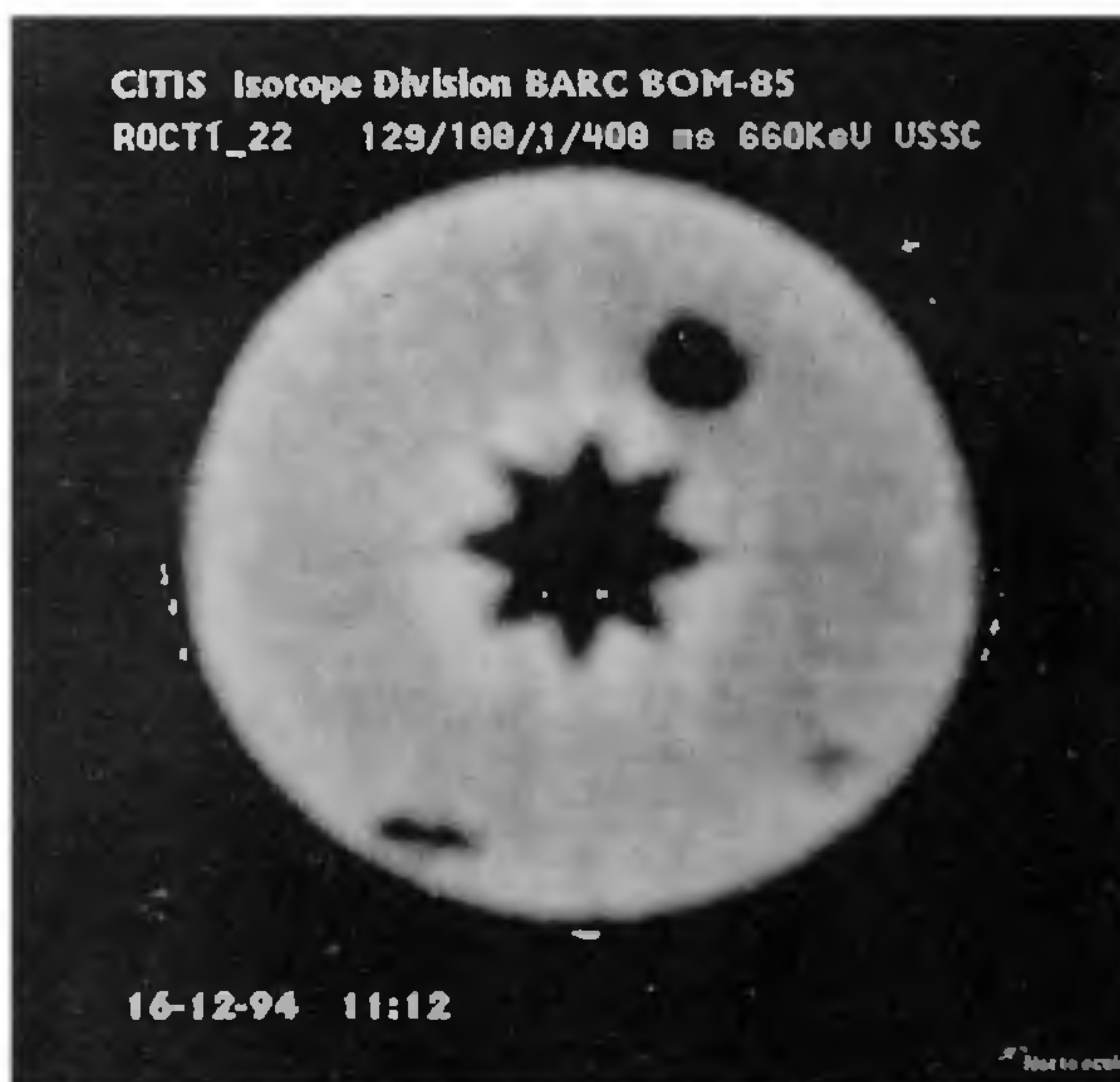
Figure 11. X-ray transmission-computed tomographs recorded and processed by G. S. Ramakrishna and colleagues in the Isotope Division of BARC, using locally-developed hardware and software.
