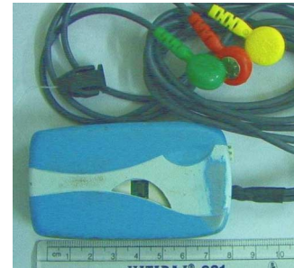
Fig. 1. A picture of the W-ECG developed at IIT Bombay, placed by the side of a 15-cm ruler.
