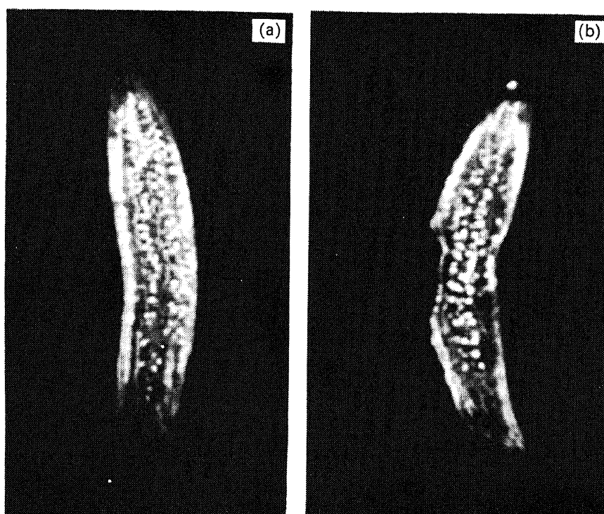
Figure 2. T_1 -weighted images of 3 mm coronal section of the slender elongated brinjal: (a) normal and (b) spoiled.
