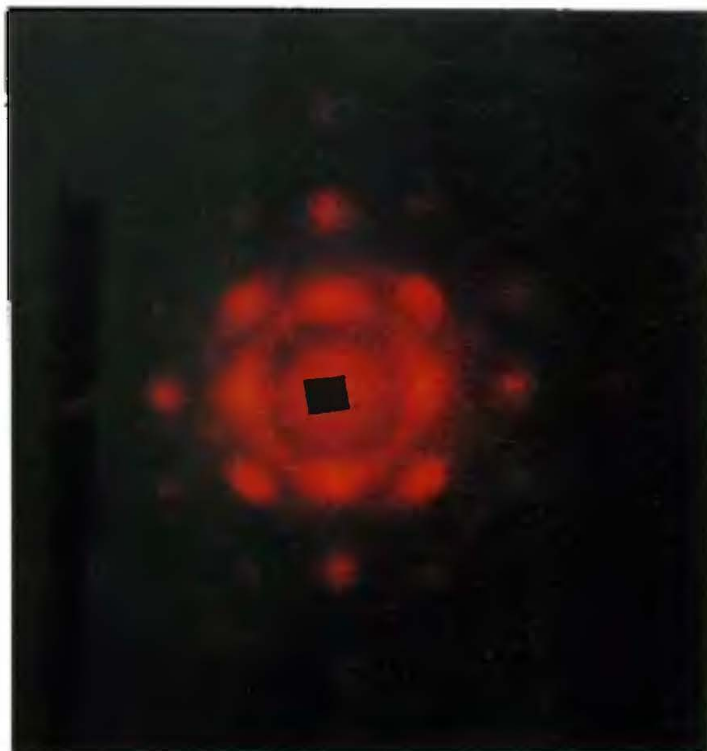
Figure 3c. Diffraction pattern of a He-Ne laser beam produced by the square lattice of the type shown in Figure 3 b.
