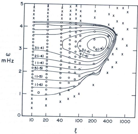
The contours of equal stability coefficient  $\eta$  are shown in the  $(\omega-1)$  diagram where the crosses (X) denote the stable modes and open circles (0) the unstable modes.
