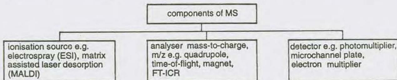
Fig. 3—Simplified schematic diagram of a mass spectrometer (MS).
