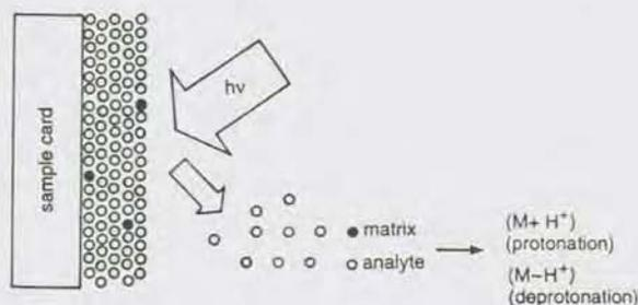
Fig. 1—Schematic diagram showing mechanism involved in matrix assisted laser desorption-ionization.
