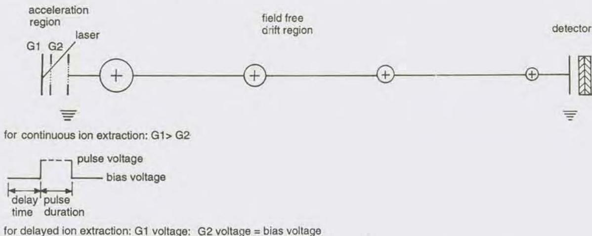
Fig. 4—Schematic representation of basic components of a linear TOF mass spectrometer.
