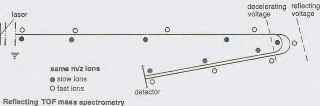
Fig. 5—Schematic representation of basic components of a reflecting TOF mass spectrometer.
