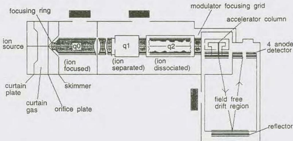
Fig. 6—Schematic diagram of quadrupole TOF instrument, representing different sections of quadrupole (modified from Mann *et al.*, 2001).
