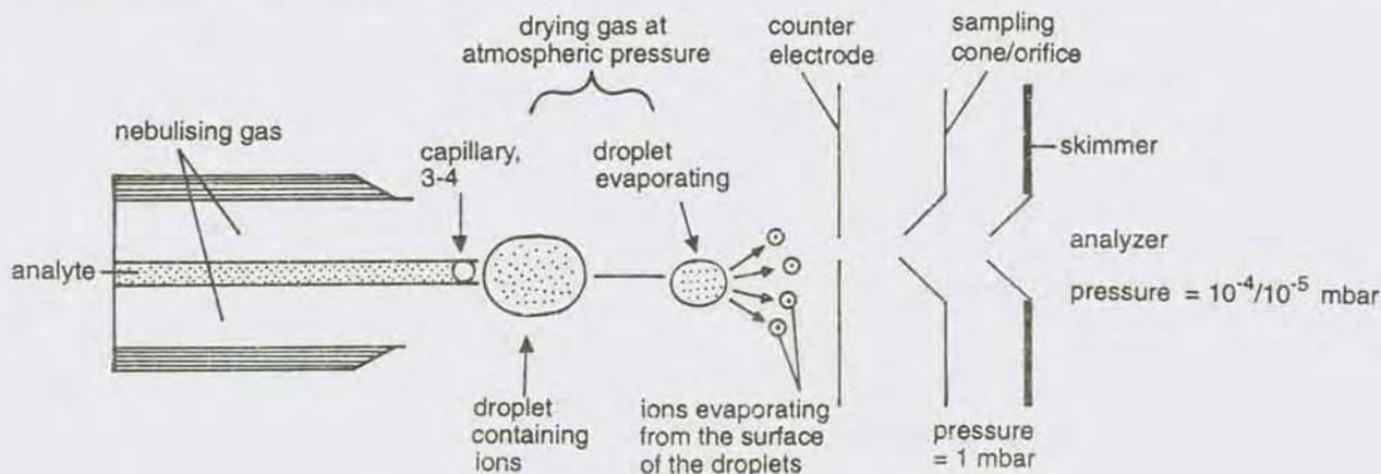
Fig. 2—Schematic diagram of standard electrospray ionization source.
