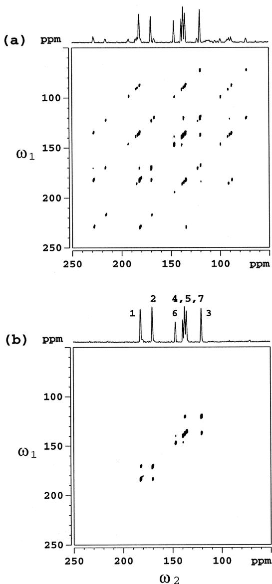
Fig. 1.  $^{13}\text{C}$  exchange spectrum of tropolone using (a) MAS at a constant spinning speed of 3.5 kHz and (b) VSMAS. In (b), the spinning speed was varied from 2 to 5 kHz in 256 regular steps of about 12 Hz after every  $t_1$  increment. Both the experiments were carried out at 315 K and use the pulse scheme  $\text{CP}-t_1(^1\text{H-decoupled})-90_{-y}-\tau-90_y-t_2(^1\text{H-decoupled})$  with recycle delay 30 s, mixing time ( $\tau$ ) 1s and TPPI phase cycle for CP.
