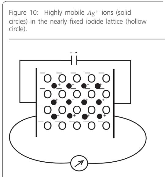
Figure 10: Highly mobile  $Ag^+$  ions (solid circles) in the nearly fixed iodide lattice (hollow circle).
