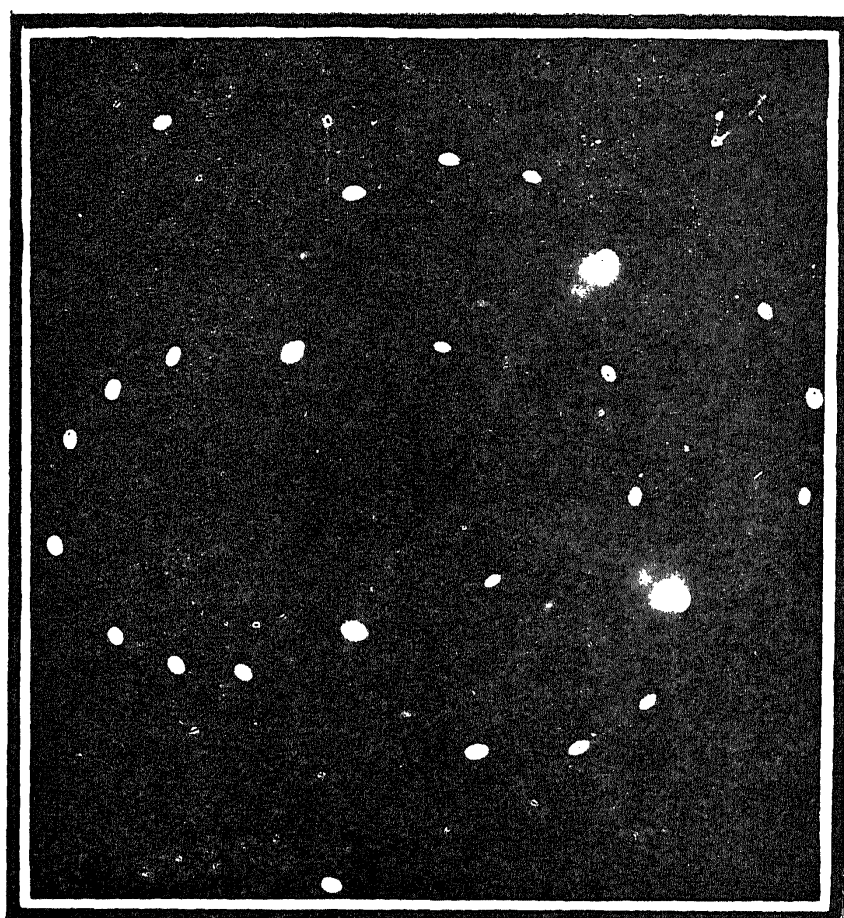
FIG. 5. Dynamic Reflections by Sodium Nitrate at 225°C. (After Raman and Nilakantan, May 1940)
