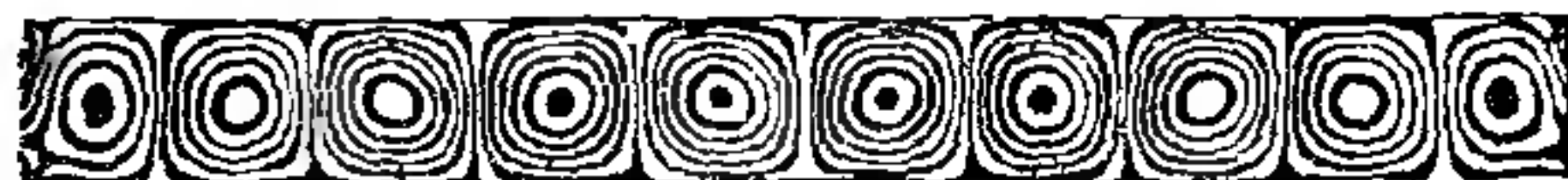
Figure 3a. Convection rolls in a horizontal layer of fluid when the lower plate is warmer than the upper plate. The curves in the diagram are density contours: In the absence of convection they would have been a series of parallel lines 1 .
