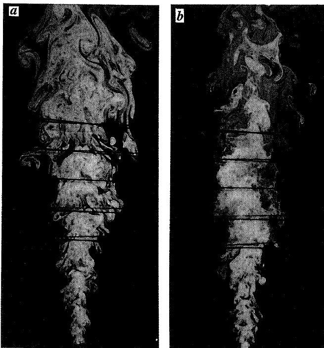
Figure 3. Vertical cross-sections of the (a) unheated and (b) heated jet at G = 1.6 .
