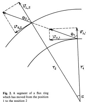
remains  $v_1$  when the ring expands to radius  $r_2$ , whereas the radius vector of the fluid particle sweeps through an angle  $\alpha$  (see Fig. 2). If  $\Delta t$  is the time taken by the ring radius to expand from  $r_1$  to  $r_2$ , then
