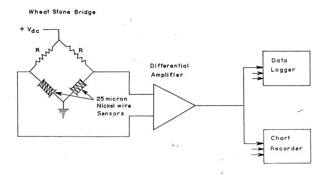
Figure 2. Block diagram of the microthermal fluctuation measurements system.
