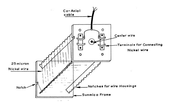
Figure 1. A microthermal sensor of the type used in the microthermal fluctuation measurements. The resistance element is shown as a spiral of 25 micron nickel wire.
