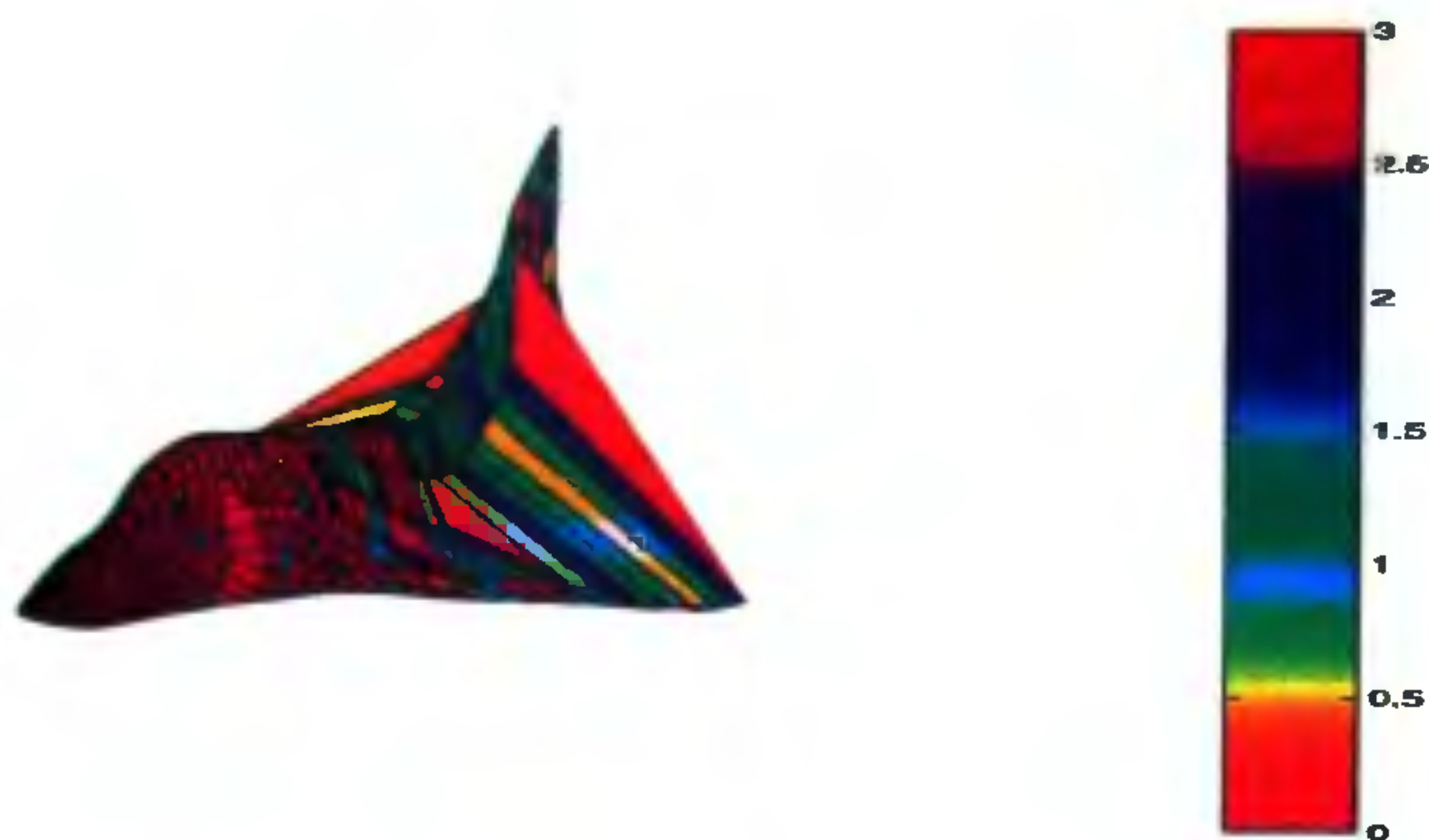
Figure 2. Current induced on an aircraft illuminated by an electromagnetic plane wave. The solution procedure generates a 2850 \times 2850 dense complex matrix.
