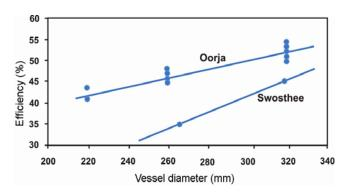
**Figure 3.** Effect of vessel diameter on efficiency, the lower plot is for the stove named Swosthee<sup>4</sup>.
