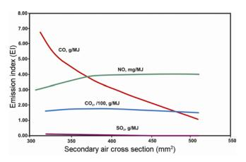
Figure 7. CO, NO and SO<sub>2</sub> emission indices with secondary air hole
