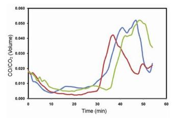
**Figure 4.** Variation of the volumetric ratio of CO: CO<sub>2</sub> during a stove operation. The operation till 30 min is in flaming mode; char mode operation begins after a short transition.
