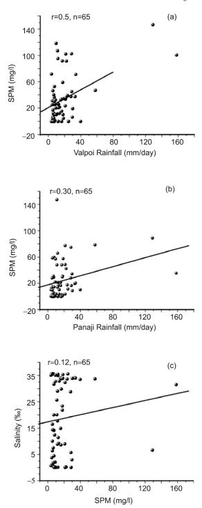
Figure 3. Scatter plots between SPM at regular station vs. rainfall (**a–b**) and, SPM vs. salinity at the regular station (**c**).
